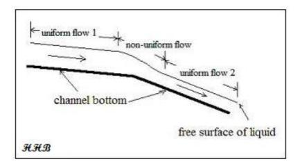
Figure 1. Uniform and Non-Uniform Open Channel Flow
