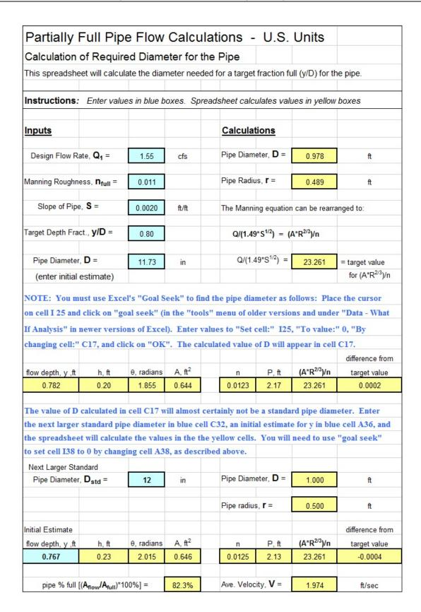
Fig. 11. Screenshot of a Spreadsheet showing the solution to Example #14
