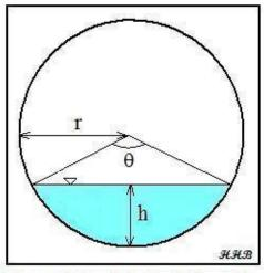
Figure 2. Partially Full Pipe Flow Parameters (Less than Half Full)
