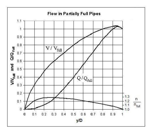
**Figure 6**. Flow in Partially Full Pipes
