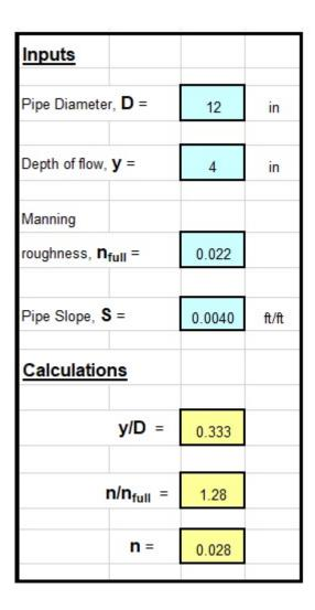
Figure 7. Screenshot for Calculation of n/n<sub>full</sub> and n for given y/D
